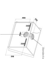
Alternative outlet: engine protrudes into the wall for 10mm
