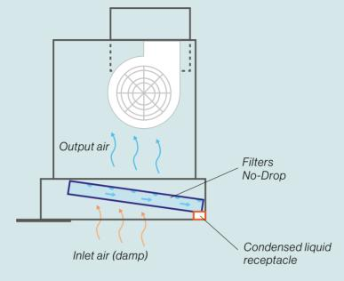
Gravity causes condensed vapours to slip along an inclined canal and flow into a receptacle for collecting liquids that can be emptied and replaced after cleaning.
